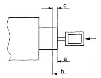
COMPONENT CHECKING AND REPAIR Checking solenoid switch Use tester to check resistance of pull-in winding (term. 50/term. 30-f). Alternator tester: 0 684 201 200 Pull-in winding resistance Starting motor - 0 001 223 0..: 0,25...0,30 Ohm Starting motor - 0 001 223 5..: 0,20...0,25 Ohm
